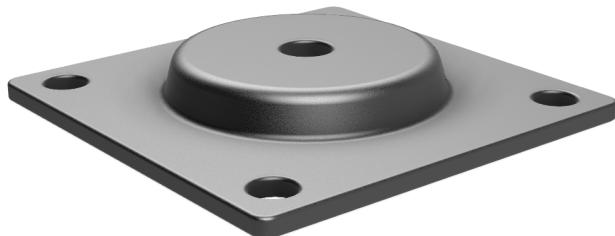
The type "M" base has been designed to provide a strong, secure mounting to any flat surface. Its application is with high strength insulators and bus assemblies, or wherever the use of a four bolt base is mandatory. Four slotted holes allow for slight field adjustment between base and mounting structure bolts. Standard base height is 1". Type "ME3" can also be used with outdoor style 3" DBC
